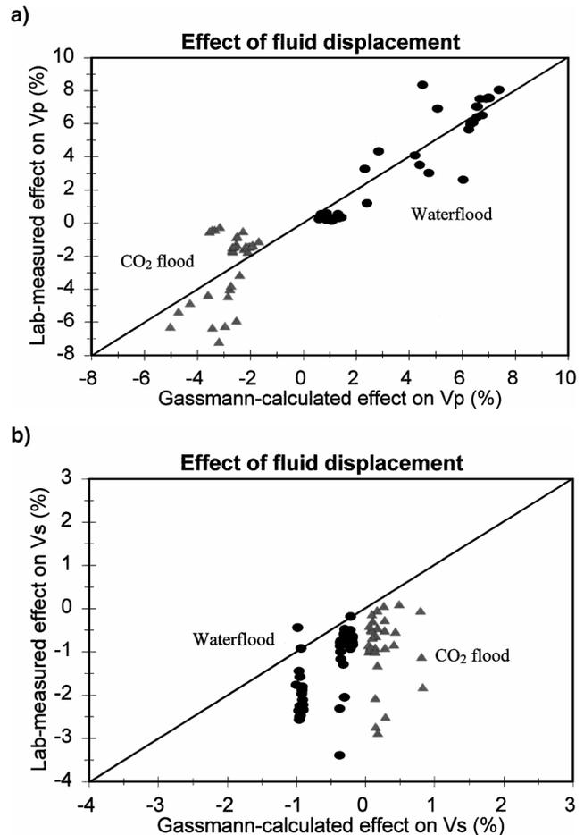
FIG. 1. Gassmann-calculated versus lab-measured effects of fluid displacement (water and CO<sub>2</sub> flood) on compressional (a) and shear (b) velocities in sands, sandstones, and dolomites. Solid circles are waterflooded sandstones and sands, triangles are CO<sub>2</sub>-flooded dolomites.
