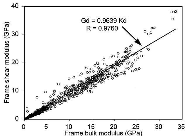
FIG. 7. A linear relationship exists between the frame bulk ( $K_d$ ) and shear ( $G_d$ ) moduli in clastic granular rocks.  $R$  is the correlation coefficient.
