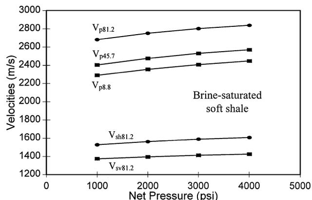
FIG. 9. Measured  $V_p$  and  $V_s$  in a brine-saturated soft shale. Three  $V_p$ 's were measured at propagation directions of 81.2°, 45.7°, and 8.8° to the symmetry axis. Two shear velocities were measured at a propagation direction of 81.2° to the symmetry axis (the  $SH$ - and  $SV$ -waves are polarized at 81.2° and 8.8° to the symmetry axis, respectively).
