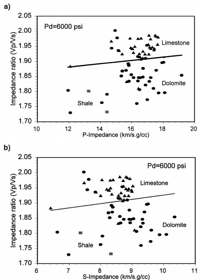
FIG. 8. Impedance ratio versus  $P$ -wave (a) and  $S$ -wave (b) impedance in carbonate rocks. A clear separation (solid line) exists between the reservoir (porous dolomite) and nonreservoir (nonporous limestone) rocks.  $P_d$  is different pressure (net overburden pressure).
