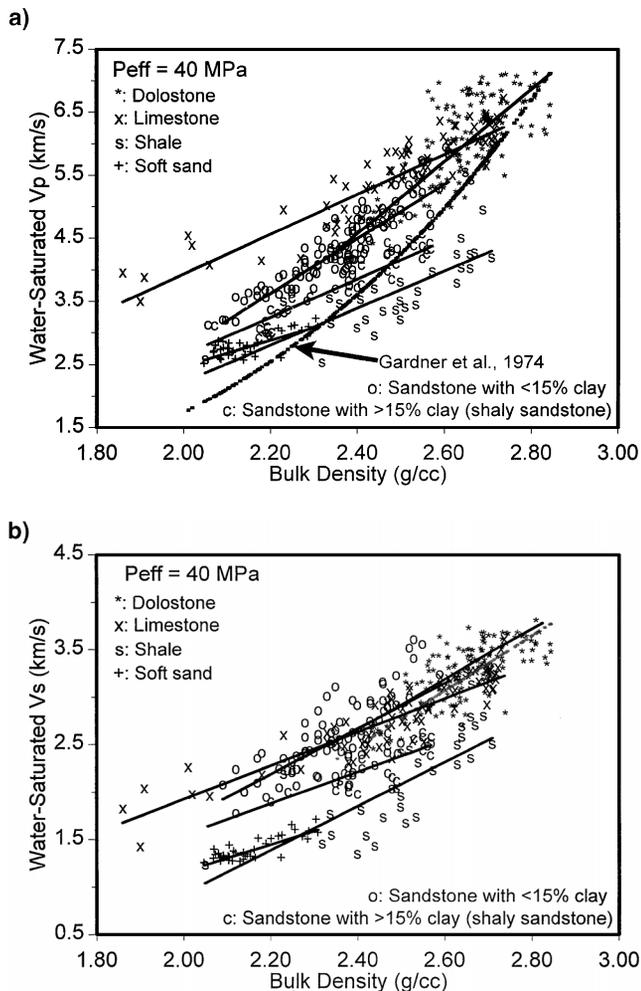
Fig. 6.  $V_p$  (a) and  $V_s$  (b) versus bulk density in sedimentary rocks. Gardner et al.'s (1974) relationship [dotted line in (a)] in general underestimates  $V_p$  in water-saturated reservoir rocks but overestimates  $V_p$  in water-saturated shales.
