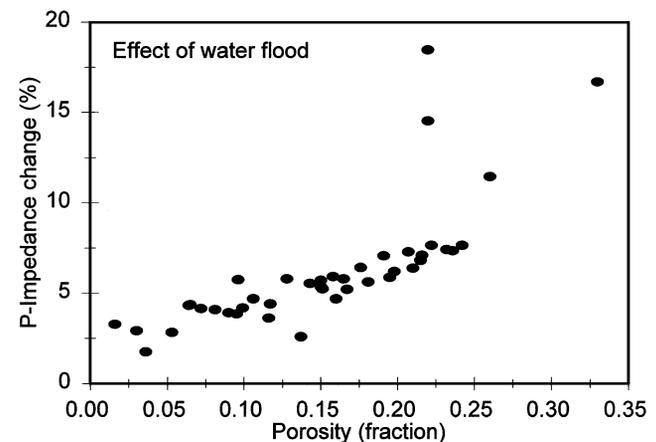
FIG. 3.  $P$ -wave impedance change as a result of water flood in 44 sandstone and sand samples versus porosity. Low porosity rocks, which tend to have hard elastic frames, show smaller effect of water flood on seismic impedances.
