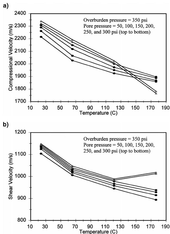
FIG. 5.  $V_p$  (a) and  $V_s$  (b) versus temperature in a heavy oil sandy. Both  $V_p$  and  $V_s$  decrease by about 15% as temperature increase from 22° to 177°C.  $V_p$  drops further between 120° and 177°C at low pore pressures (50 and 100 psi) as water inside the rock transforms to steam [the top two curves in (a)], adding another 10% or so  $V_p$  decrease. In contrast,  $V_s$  increases by about 5% as results of steam.
