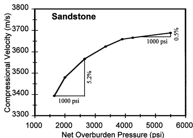
**FIG. 4.**  $V_p$  versus net overburden pressure in a sandstone. Increasing the net overburden pressure from 1650 to 2650 psi causes a 5.2%  $V_p$  increase, whereas the same amount of net overburden pressure increase from 4500 to 5500 psi only results in a 0.5%  $V_p$  increase.
