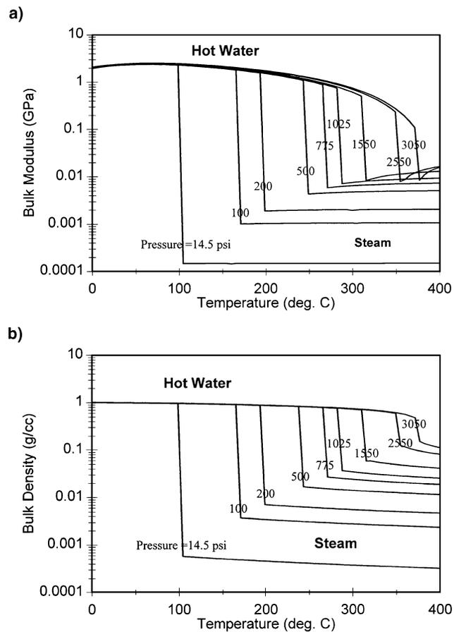
FIG. 2. Adiabatic bulk modulus (a) and density (b) of water and steam versus temperature and pressure. Both bulk modulus and density drop sharply as water transforms to steam.
